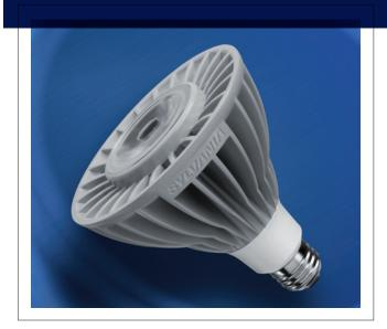
LED technology reduces energy and maintenance costs when compared with conventional light sources. Lasting 20 times longer and with only 18 watts, LED PAR38 lamps are high-quality replacements for 75W halogen PAR38 lamps. They are free of UV and IR radiation, minimizing discoloration and fading of materials. These lamps are dimmable down to 10%\* and are rated at 50,000 hours life with a correlated color temperature (CCT) of 3000K. They are available with 25° and 40° beam angles.
