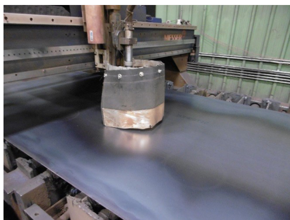
Figure 1. Factory-designed welding curtain on the south PAC system. The welding curtain covers 180 degrees of the arc. The PAC system is not operating in the photo. Photo by NIOSH.
