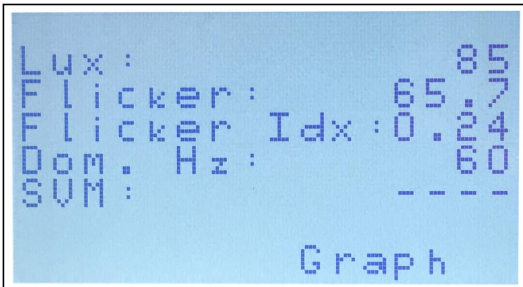
NOTE: Flicker, Flicker Idx and Dom. Hz measurements are only available when the illuminance is greater than 5 lux. SVM measure measurements are only available when the dominant frequency (Dom. Hz) is greater than 80Hz and the illuminance is greater than 100 lux.
