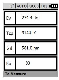
To scroll through the screens of data, use the up and down toggle buttons located below the display. Below is an example of the available data fields, Unpopulated (before measurement).
