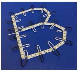
EZ flx cut and formed to the letter "B", wire can be trimmed from none divided segments
