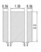
2. Dimensions in mm. Tolerance <u>+</u>.2 mm
