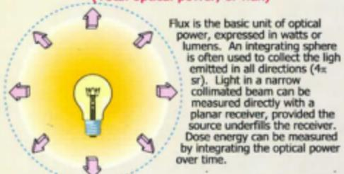
Flux is the basic unit of optical power, expressed in watts or lumens. An integrating sphere is often used to collect the light emitted in all directions ( $4\pi$  sr). Light in a narrow collimated beam can be measured directly with a planar receiver, provided the source underpins the receiver. Dose energy can be measured by integrating the optical power over time.
