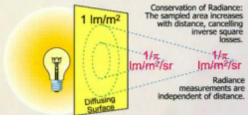
1 lux ( $1 \text{ lm/m}^2$ ) of illuminance on a perfectly diffusing surface produces 1 apostilb ( $1/\pi \text{ lm/m}^2/\text{sr}$ ) of luminance. Similarly, 1 foot-candle ( $1 \text{ lm/ft}^2$ ) will result in 1 foot-lambert ( $1/\pi \text{ lm/ft}^2/\text{sr}$ ).
