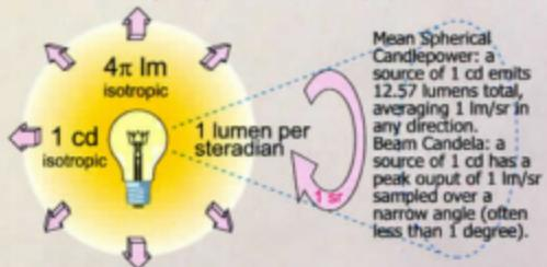
1 cd (MSC) = 1 cd (Beam) for an isotropic source. A 1 cd (MSC) laser beam may have 1,000,000 cd (Beam) output.
